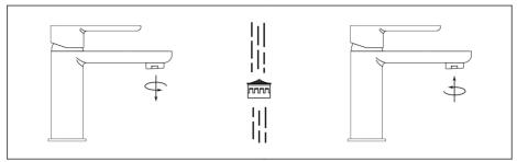
Periodically the aerator will need to be cleaned. Using an aerator key, remove the aerator from the spout, flush the aerator under water to remove the small debris or soak overnight. Re-install the aerator back into the tap and re-tighten.
