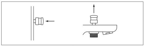
All diverters only function when the main water supply is turned on, for concealed shower valves push the button in to divert and for deck/floor mounted bath/shower mixers pull the diverter knob
