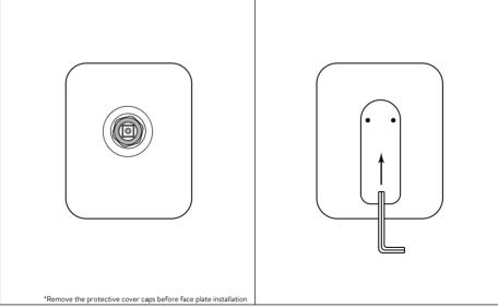
Apply the surrounding finishes, fit the face-plate onto the valve body.
