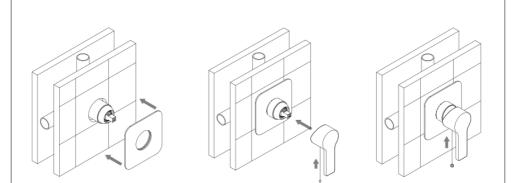
Once the surrounding finishes have been applied (Tiles/Marble etc.) remove the protection covers. Fit the face plate onto the mixer body, it is advised to use a small amount of lubricant on the rubber seals. Slide the handle onto the cartridge pin and secure with the grub screw, then push on the cover cap.
