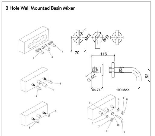
Assemble the parts as per the diagram. Ensure that the mains water supply is turned off before installation.
