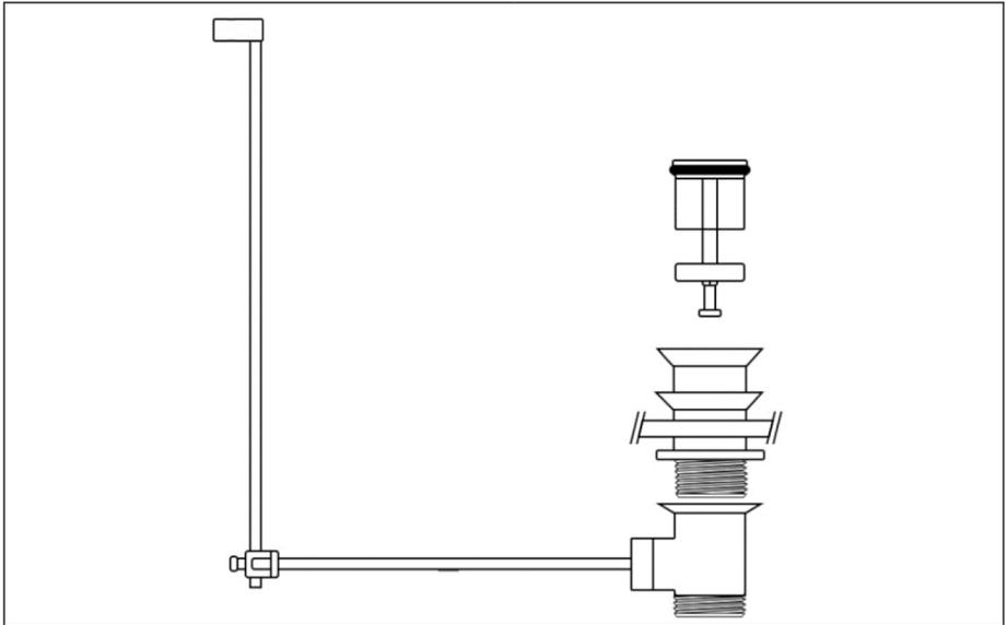
Disassemble the pop-up waste and reassemble onto the basin ensuring the foam washer is placed between the top waste housing and the basin. The rubber washer is to be placed on the bottom waste housing before being tightened
