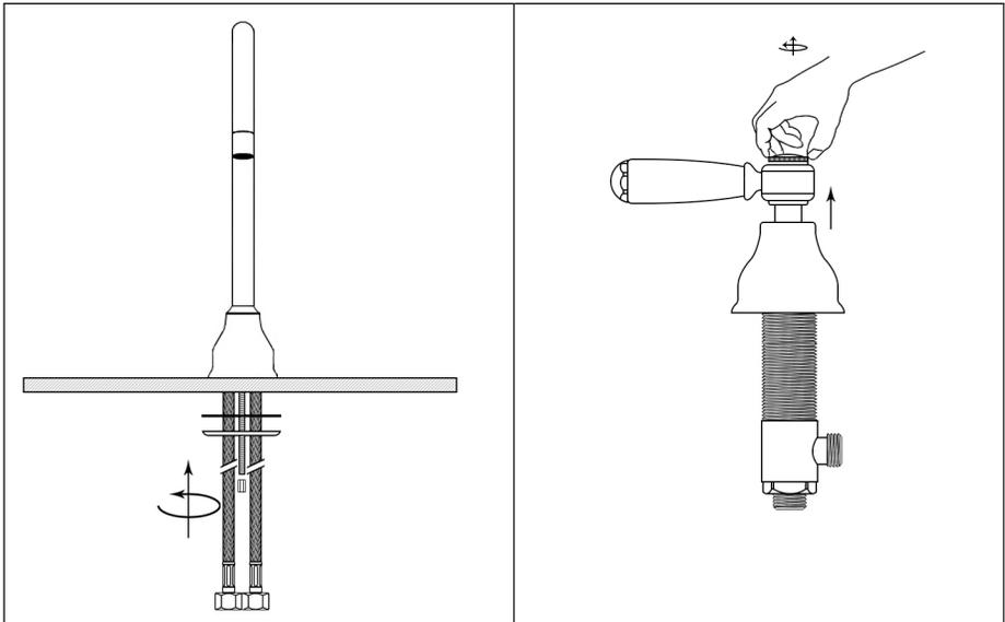
Slide the rubber 'C' washer followed by the metal 'C' washer and tighten the back nuts with a spanner to secure the spout.
