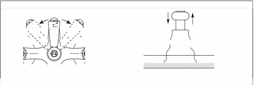
All diverters only function when the main water supply is turned on, for exposed bath/ shower mixers lift the diverter lever to left for the spout and right for shower, for deck mounted bath/shower mixers pull the diverter knob.
