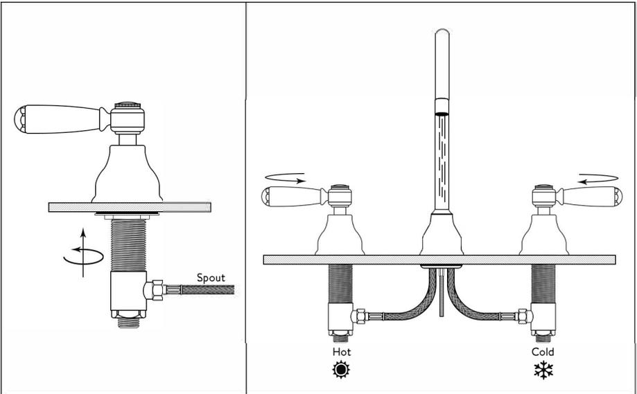
Then tighten to clamp the valve to the basin/counter with the back nuts, being careful not to over tighten. Connect the flexible hose from spout to the valve.
