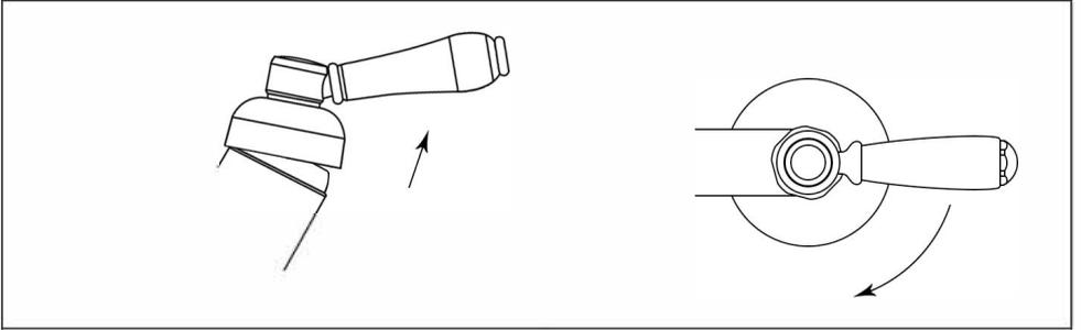
To control water flow on deck mounted mono mixers lift the handle upward, push down for valved mixers. To adjust the temperature for mono lever mixer, turn the handle to the right for cold water and left for hot water
