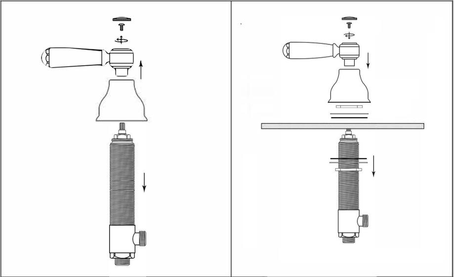
Remove the screw to separate the valve body, shroud and handle as shown above.
