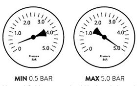
Hot and Cold pressure should be kept balanced within 1 BAR
