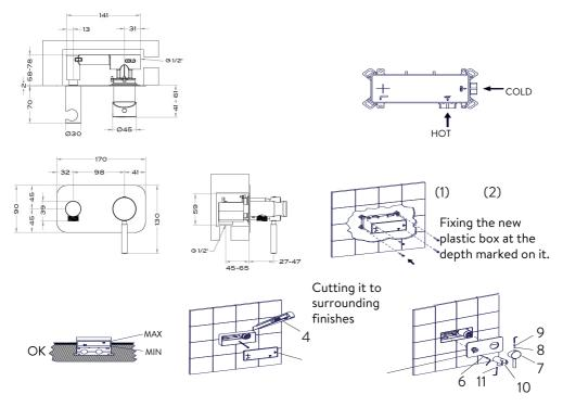
Assemble the parts as per the diagram.
