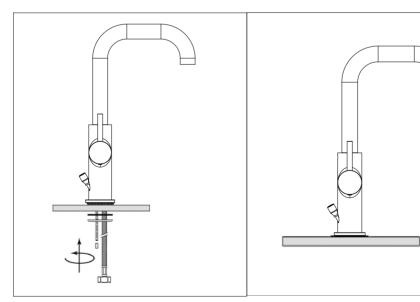
Slide the rubber 'C' washer followed by the metal 'C' washer and tighten the back nuts with a spanner to secure the mixer.
