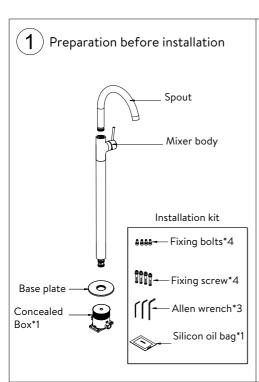
Make a slot underground size must over 120 x 130 mm, depth 70-100mm including the upper brick.
