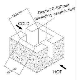
3 Connect the concealed valve with plumbing, open the valve and get the leakage test done properly.
