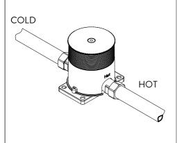
Drill installation holes in the bottom (Ø8mm×4), then install the fixing bolts into the holes.
