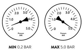
Hot and Cold pressure should be kept balanced within 1 BAR
