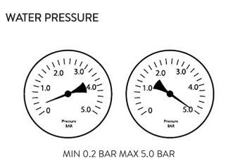
Hot and Cold pressure should be kept balanced within 1 BAR
