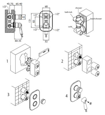
Assemble the part as per the diagram.
