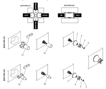
Assemble the part as per the diagram.
