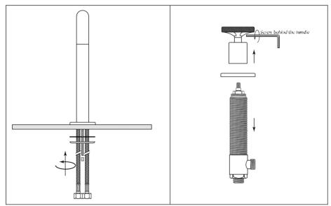
Slide the rubber 'C' washer followed by the Installation of Valve. metal 'C' washer and tighten the back nuts with a spanner to secure the spout.
