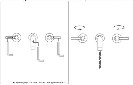
Install the face plates, then slide the spout into the spout connector, Install the handles secure all by tightening the grub screws.
