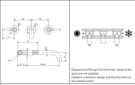
Install the concealed parts at a depth so that Install the cold water supply from the that finished surface is between the Min/Max markings shown above.
