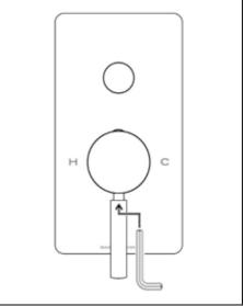
Install the handle onto the cartridge pin And secure by tightening the grub screw. Turn on the water and test the mixer.
