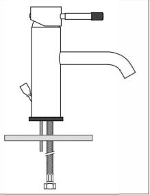
Install the threaded rods and hand-tighten the flext-pipes into the bottom of the mixer body.
