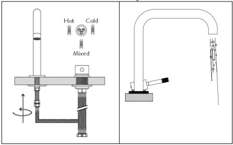
Install the mixed water flexible to the spout nut connection.
