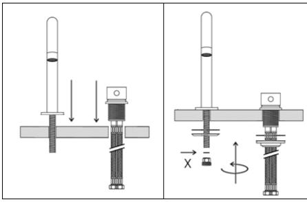
Feed the two pre-assembled components through the holes in the basin/countertop.
