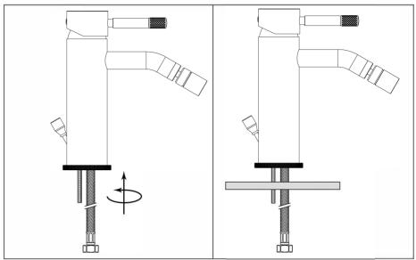
Install the threaded rods and hand-tighten the flext-pipes into the bottom of the mixer body.
