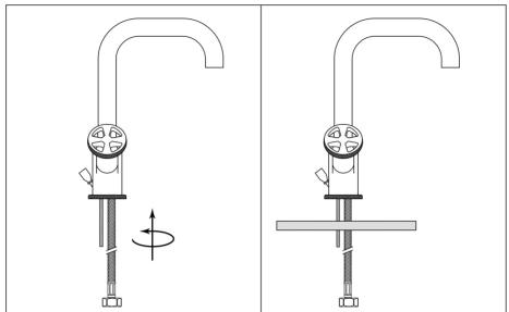
Install the threaded rods and hand-tighten F the flext-pipes into the bottom of the mixer b body.
