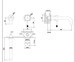
Assemble the part as per the above. Ensure that the mains water supply is off before installation. Install the mixer housing (1) at a depth so that the finished surface is between the Min/Max distance in the drawing.
