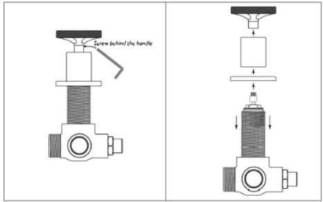
Installation of diverter. Loosen the screw (behind the handle knob) with an allen key.
