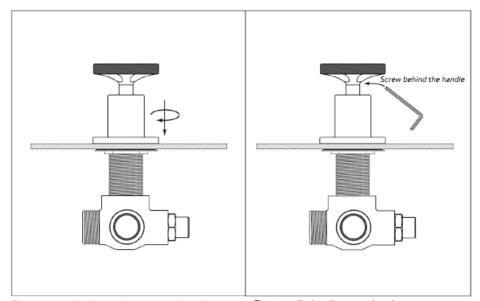
First screw the base plate onto the diverter top, then from underneath tighten the back nut up to secure.
