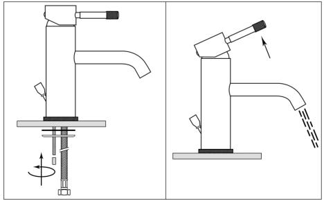
Slide the rubber 'C' washer followed by the Flush the pipework, then connect the fleximetal 'C' washer and tighten the back nuts with a spanner to secure the mixer.
