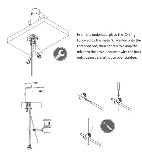
Install the waste ensuring that the foam washer is in between the waste and the basin on the top portion of the waste, the rubber washer is to be placed under the basin before the bottom part of the waste is connected and tightened up. Again take care not to over tighten.
