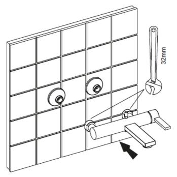
Place the 'O' rings into the nut connections and tighten to the eccentrics.
