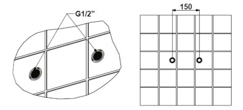
Pre install  $2x \frac{1}{2}$ " female fittings into the wall, these fittings should be flush to the finished wall surface.
