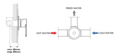
Install the mixer housing at a depth so that the finished surface is no further than the maximum distance marking shown in the diagram.
