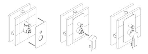
Once the surrounding finishes have been applied (Tiles/Marble etc.) remove the protection covers. Fit the face plate onto the mixer body, it is advised to use a small amount of lubricant on the rubber seals. Slide the handle onto the cartridge pin and secure with the grub screw, then push on the cover cap.
