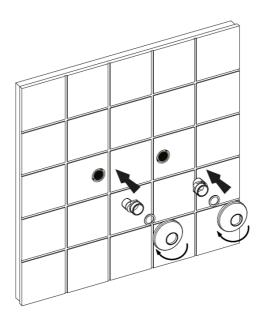
Wrap the 2 eccentrics with PTFE tape and install into the wall provisions, making sure the eccentrics are level and are the correct distance apart. Screw on the cover shrouds until secure against the wall surface.
