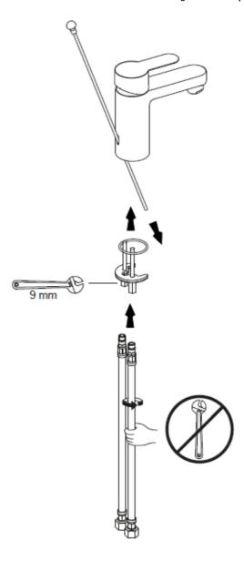
Place the threaded rods and 2 flexible pipes into the body of the mixer. Insert the push rod through the hole in the mixer body. place the assembly through the basin / counter making sure to install the base ring and washer.
