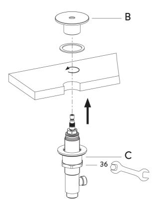
Fit the two standings, fitting it from below and screwing the chrome ring (B) with its gasket, and fix the set with the fixing nut (C).
