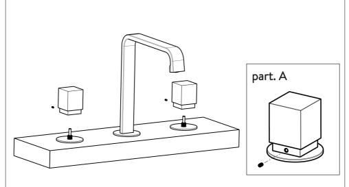
Finally fit the two handles and fix them with their grub screws (see part. A).
