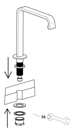
Fit the spout fixing the set with the lower fixing nut and gaskets.
