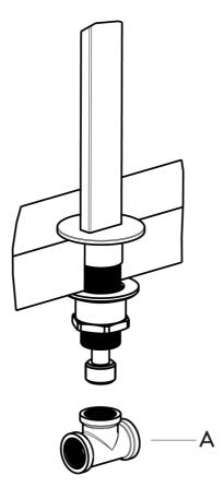
Fit the T connection (A) by screwing it to the lower side of the spout. We suggest to adjust it in the right position to fit then the two taps at its sides.
