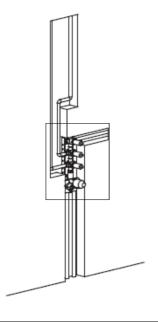
Pull out th jackets, & install the panel, female thread sockets, hand wheels and other parts.
