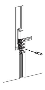
Turn on the valve and observe for 5-10 minutes, check whether the connections are tight and make sure there is no leakage or seepage, and then turn off the valve. Fix the control valve. Fix the valve in the slot using self-tapping screws and plastic expansion plugs.
