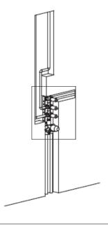
Pull out th jackets, & install the panel, female thread sockets, hand wheels and other parts.
