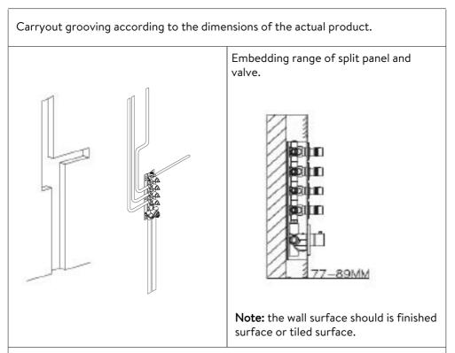
Take out the hand wheels, female thread sockets, panel and PVC pipes, and then install the 52 jacket and 30 jackets.
