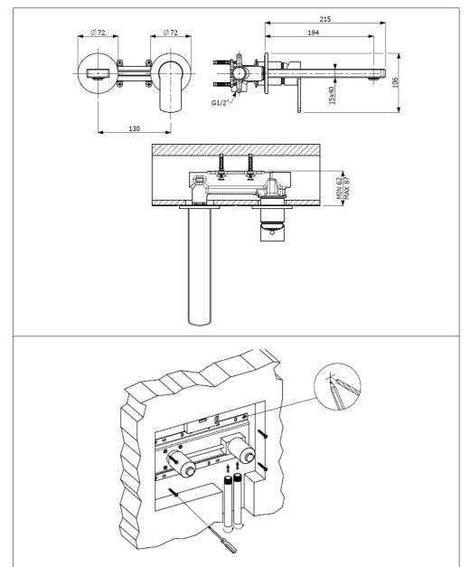
Install the mixer housing (1) at a depth so that the finished surface is between the Min/Max distance markings shown in the diagram. Mark the holes on the fixing bracket.
