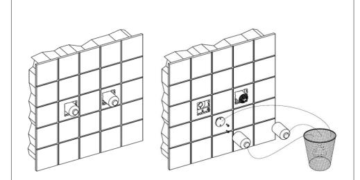
Remove the cap & place on the protection covers.
