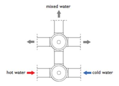
Connect the Hot and Cold water supplies to the mixer, then install the mixed water supply, cap off and pressure test to check for any leakage\*
