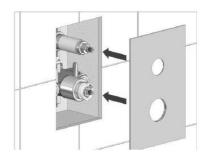
Screw the adapter (2), or the adapters, with their O-ring (1), until the plate is against the wall.
