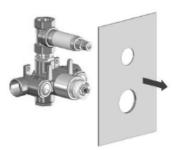
Unscrew the threaded rod with a 17mm wrench.
