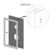
Fix the cover plate over the temperature valve and the threaded rod
