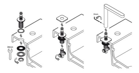
Install the spout body into the basin/countertop, from underneath fasten by using the rubber washer, metal washer and back-nut. After this is secure place the cover plate over the spout body.
