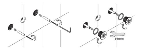
Install the spindle extensions and tighten with the scres and Allen key, Place the shrouds over and tighten into the mixer housing.
