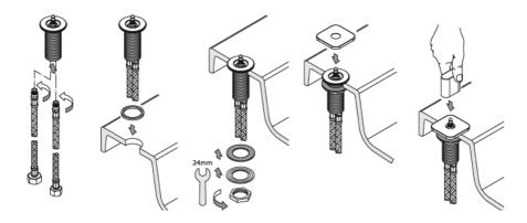
Install the flexible pipes into the valve body. Then place this assembly through the basin/countertop, from underneath fasten by using the rubber washer, metal washer and back-nut. Place on the base plate, then press on the handle, repeat for the other valve.
