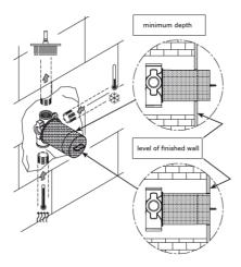
Install the mixer housing at a depth so that the finished surface is between the Min/Max distance markings shown on the diagram.
