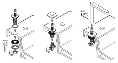
Install the spout body into the basin/countertop, from underneath fasten by using the rubber washer, metal washer and back-nut. After this is secure place the cover plate over the spout body.
