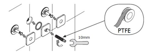
Wrap the required amount of PTFE tape onto the spout connection, place through the back plate and tighten into the mixer housing, place the 2 back plates over the spindle extension.
