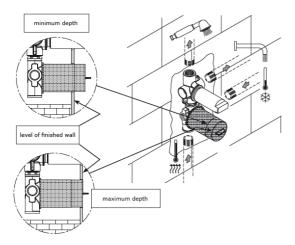
Install the mixer housing at a depth so that the finished surface is between the Min/Max distance markings shown on the diagram.
