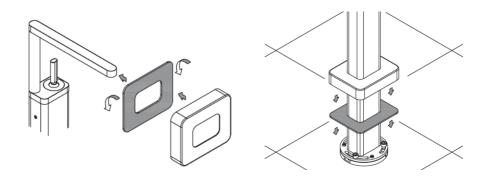
Carefully place the washer and base cover over the mixer and slide down to the base of the mixer
