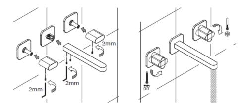
Install the 2 handles and the spout and tighten from the underside with the grub screws and Allen key.
