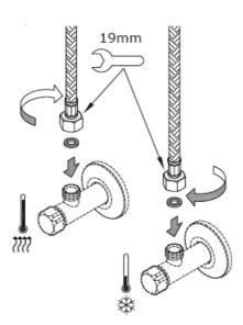
Install the flexible pipes, onto the water supply valve. Open the water supplies and test for leaks on the connections.
