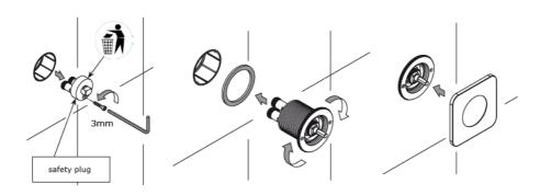
Remove the safety plug using the Allen key, insert the cartridge and rotate the the shroud until tight. Place the face plate over the shroud.
