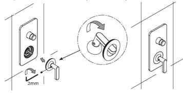
Loop the ring over the handle and insert on to the spindle, tighten using the Allen key.
