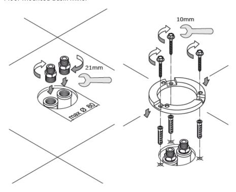
The mixer requires pre-installed pipework terminating with ½" female sockets at finished floor level.
