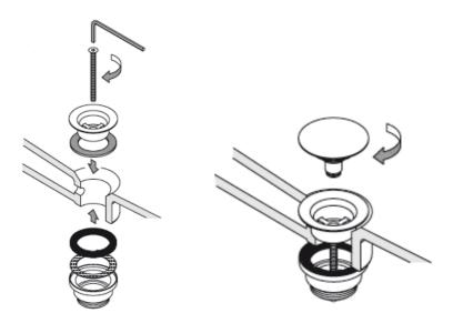
Install the waste waste housing as per the above, being careful not to over tighten. Then screw in the push type waste into the housing. And test for functionality.
