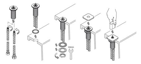
Install the flexible pipes into the valve body. Then place this assembly through the basin/countertop, from underneath fasten by using the rubber washer, metal washer and back-nut. Place on the base plate, then press on the handle, repeat for the other valve. Follow the same process for the diverter D
