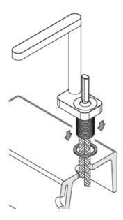
Now place the assembly onto the basin / counter, making sure to insert the washer.
