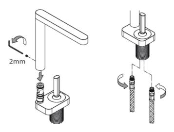
Place the spout over the outlet and tighten with the grub screw. Then insert the two flexible pipes into the mixer body.
