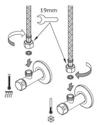
Install the flexible pipes, onto the water supply valves
