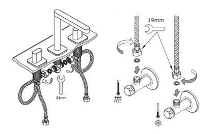
Connect the valve water flexibles to the spout,
