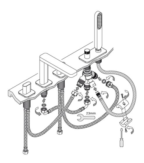
Install the valve flexibles into the right and left side of the diverter valve, install one hose from the bottom of the diverter valve to the spout. Install the handshower hose into the angled female connection. Plaese make sure to use 'O'rings on all connections. Lastly attach the hose weight to the shower hose.
