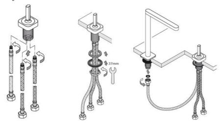
Install the hot, cold and mixed water flexible pipes into the mixer body. Then place this assembly through the basin/countertop, from underneath fasten by using the rubber washer, metal washer and back-nut.
