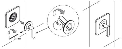
Loop the ring over the handle and insert on to the spindle, tighten using the Allen key.
