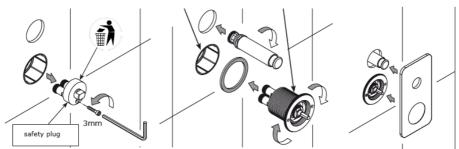
Remove the safety plug using the Allen key, insert the cartridge and rotate the the shroud until tight, install the diverter and place the face plate over the shroud.
