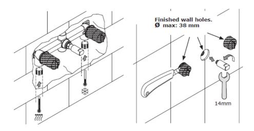
Install the mixer housing at a depth so that the finished surface is no more than the Max distance markings shown in the diagram. Connect the Hot and Cold water supplies to the mixer and cap off the outlet connection, pressure test to check for leaks at the connections.
