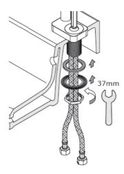
From the underside, place the 'O' ring followed by the metal washer onto the threaded rod, then tighten the nut to clamp the mixer to the basin / counter with the back nut, being careful not to over tighten.
