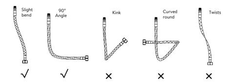
Important: Failure to follow these guidelines may result in poor perfor-mance and damage to the flexible connecting pipes.
