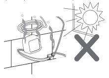
The adaptor can't be installed in wet surroundings.
