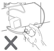
Any operation is disallowed when adaptor is connected to power
