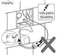
The size of cable should be 1.0-2.5mm<sup>2</sup> and the wire connector should be connected firmly.
