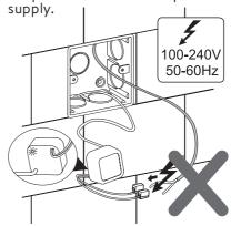
The size of cable should be 1.0-2.5mm and the wire connector should be connected firmly.
