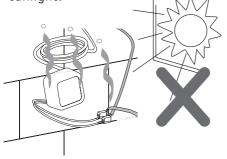
The adaptor can't be installed in wet surroundings.  $\lambda$
