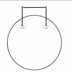
To use the measure tape to measure the distance between the two holes.
