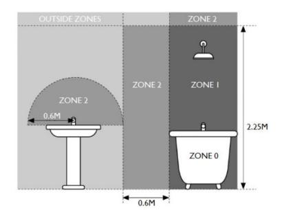
Zone 0 is inside the bath or shower tray itself. Any appliance used in this zone must be rated at least IP67 which is total immersion proof.
