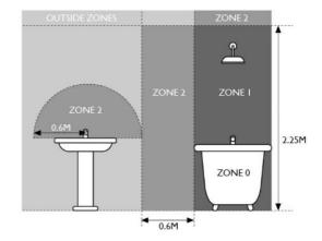
Zone O is inside the bath or shower tray itself. Any appliance used in this zone must be rated at least IP67 which is total immersion proof.
