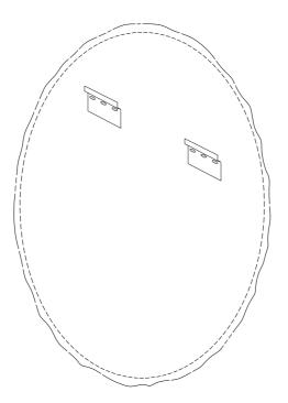
On the reverse side of the mirror check the type of fixing point required to hang the mirror, also check the correct orientation.
