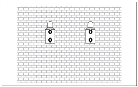
Screw the brackets to the wall.
