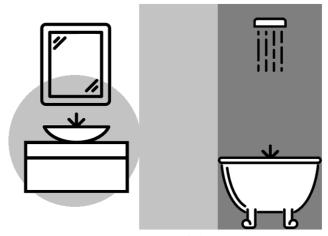
Zone 0 is inside the bath or shower tray itself. Any appliance used in this zone must be rated at least IP67 which is total immersion proof.
