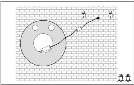
2 persons may be required to hang the mirror, place the mirror above the brackets, then slowly slide down, the mirror can be slightly pivoted to allow vision of the brackets. Ensure the wire isn't caught or kinked as its hung.
