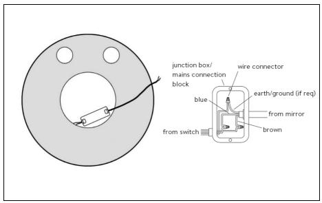
Allow plenty of wire flex from the wall to a place where the mirror can comfortably sit, connect the live and neutral wires into a suitable junction/mains connection block.
