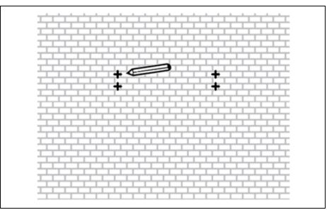
Measure the distance between the brackets on the rear-side of the mirror, Calculate this distance into the final position of where the mirror will be hung, and mark the 2 points on the wall.
