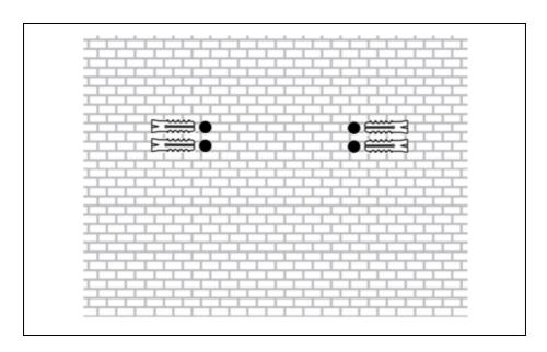
Insert the plugs into the wall, if slightly tight, tap in with a hammer.
