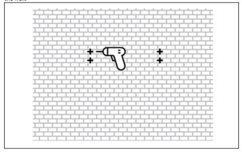
Drill the two marks to the depth of plug that will be used.
