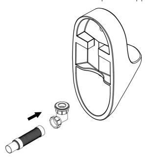
After installing urinal waste install the urinal spreader & connect the hose to the spreader.
