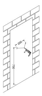
Push plastic fisher wall plugs into wall then install the Urinal fixing Bracket with flat head screws.
