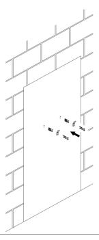
Carefully lift the urinal & install the Urinal waste trap and waste pipe.
