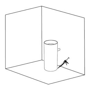
Finalise the position of the basin and run a small bead of silicon around the perimeter base.
