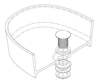
Install the waste into the basin and connect the bottle trap. If required use a flexible waste pipe from the bottle trap to the wall outlet.
