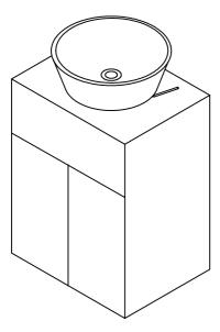
PLACE THE <u>BASIN</u> ON THE UNIT WORK TOP, MARK AROUND THE BASE, POSITION OF THE WASTE AND ANY TAP HOLES IF REQUIRED.
