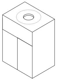
CUT OUT FOR THE WASTE ALLOWING FOR ACCESS (APPROX 120 mm DIA) MAKING SURE THE CUT OUT IS NOT VISIBLE WHEN THE BASIN IS IN PLACE. ALSO CUT OUT FOR ANY TAPS AND CONNECTIONS IF REQUIRED. ENSURE ALL CUT EDGES ARE SEALED AGAINST WATER INGRESS.
