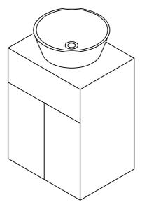
PLACE THE <u>BASIN</u> INTO POSITION ON THE WORK SURFACE AND PRESS DOWN TO MAKE A SEAL.CLEAN OFF ANY EXCESS SEALANT AND FINISH ACCORDINGLY.
