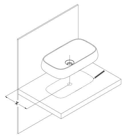
Place the basin on the counter-top, take notice of the spout length of the mixer so that the distance X is correct. Mark around the perimeter of the basin and waste hole.
