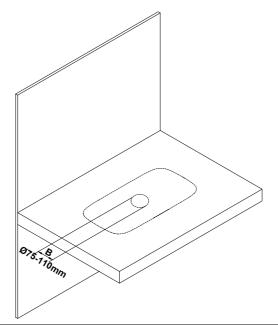
Install the waste assembly into the basin.
