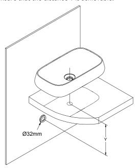
Drill waste hole allowing for the finished dimensions of the waste outlet. In this instance its B=75-110 mm, please check your corresponding waste outlet product.
