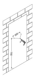
Push plastic fisher wall plugs into wall then install the L-Bracket with screw.
