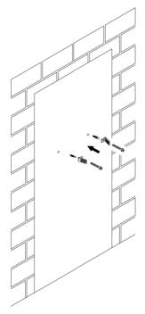
Carefully lift the urinal & install the urinal spreader and urinal waste. connect the hose to the spreader. Form a U bend in the flexible waste so that have at least a 75mm trap seal.
