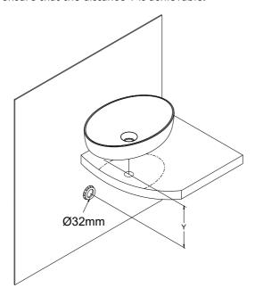
Drill waste hole allowing for the finished dimensions of the waste outlet. In this instance its B=75-110 mm, please check your corresponding waste outlet product.
