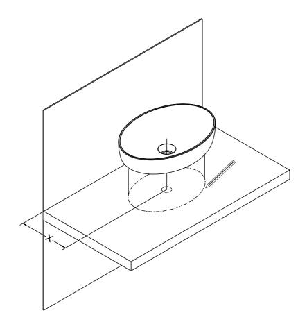
Place the basin on the counter-top, take notice of the spout length of the mixer so that the distance X is correct. Mark around the perimeter of the basin and waste hole.
