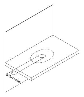
Install the waste assembly into the basin.
