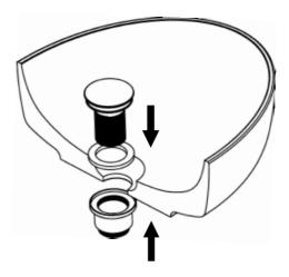
If required, place a few dots of silicon on the base of the basin, align, and place in position, allow the silicon to cure for a few hours.
