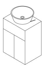
PLACE THE BASIN ON THE UNIT WORK TOP, MARK AROUND THE BASE, POSITION OF THE WASTE AND ANY TAP HOLES IF REQUIRED. 2
