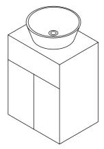
PLACE THE BASIN INTO POSITION ON THE WORK SURFACE AND PRESS DOWN TO MAKE A SEAL.CLEAN OFF ANY EXCESS SEALANT AND FINISH ACCORDINGLY.
