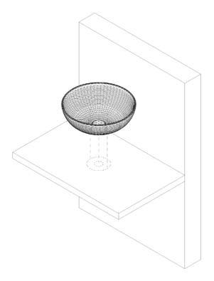
If required, place a few dots of silicon on the base of the basin, align, and place in position, allow the silicon to cure for a few hours.
