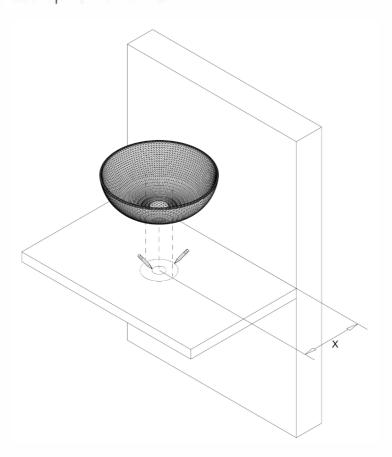
P ace the basin on the countertop, take notice of the spout length of the mixer so that the distance X is correct. Mark around the perimeter of the basin and waste hole
