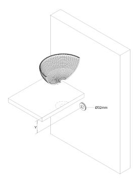
Check that the waste provision is in the correct place, check the bottle trap dimensions to ensure that the distance Y is achieveable.
