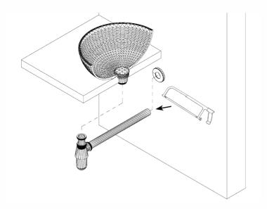
Install the bottle trap onto the waste, cut the horizontal pipe to length and install into the wall via a waste compression fitting or rubber socket.
