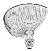
Install the waste assembly into the basin.
