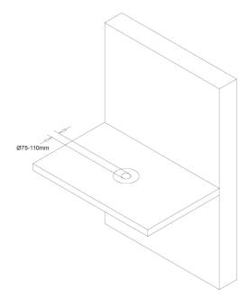
Drill waste hole allowing for the finished dimensions of the waste outlet. In this instance its 075-110mm, please check your corresponding waste outlet product.
