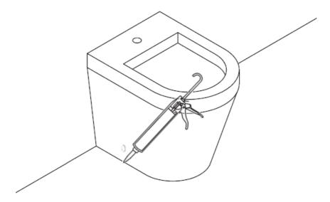
Clean away the pencil lines and place a small bead of silicon around the bidet
