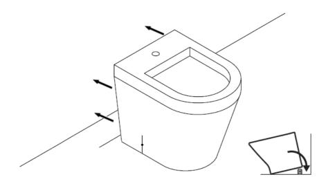
Carefully lift the bidet over the fixing kit, then slide the bidet backward guiding the waste pipe into the wall outlet connection before fully pushing back to the wall, this should now line up with the existing drawn lines.
