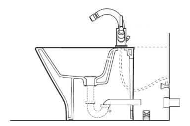
Install the desired **BAGNODESIGN** bidet mixer and waste, connect the supplies to the angle valve, turn on and test for leaks. Connect the bottle trap to the waste, align the pipework to the wall outlet.
