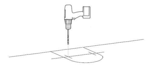
Remove the bidet from position and turn over, measure the thickness of the ceramic, add this dimension across the parallel lines. Where the 2 lines meet carefully drill and plug the holes.
