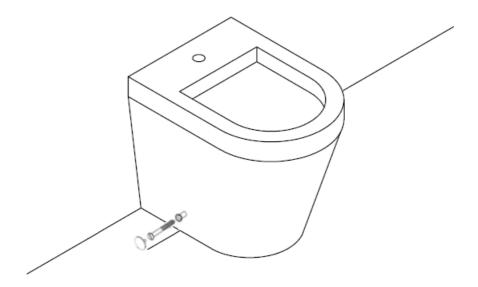
Secure the bidet to the fixing kit with the plastic sleeves and the screws. Fit the plastic cover caps over the heads of the screws.
