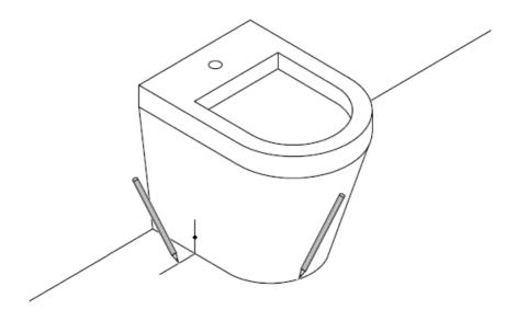
Place the bidet in position and draw around the base perimeter. Also draw a line parallel to the fixing holes.
