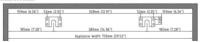
NOTE: If the appliance is relocated, the bracket must be removed and installed in the new location.
