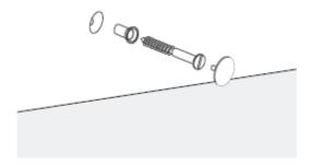
Install the rubber sleeve through the screw and tighten to the side of the WC. Simply then push the screw cap over to complete.
