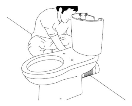
Place the WC in final position and attach water and waste connections. This would be a good time to check the assembly for leakages.
