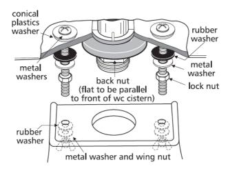
Push sponge close coupled washer onto back-nut, this will ensure centralization before assembling to the WC pan.
