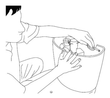
Mark the two wall fixings (if applicable) inside the cistern ensuring that the assembly remains level. The Close coupled WC can then be removed from desired position.
