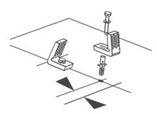
From the base mark line, measure in 30-40mm, and draw a line connecting the two side fixing hole positions. Carefully drill and plug.
