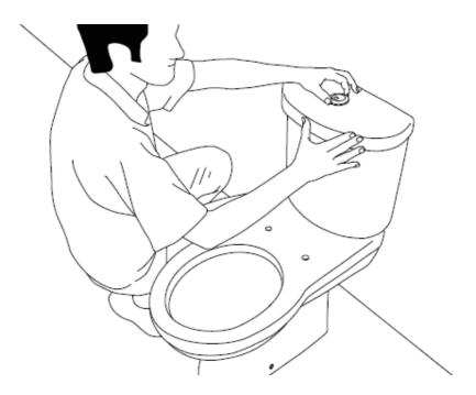
Place the cistern lid on to the cistern and screw the push button assembly until tight. This now successfully completes the Close-Coupled WC
