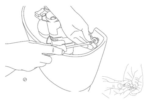
Screw the cistern body to the wall using the appropriate fixings
