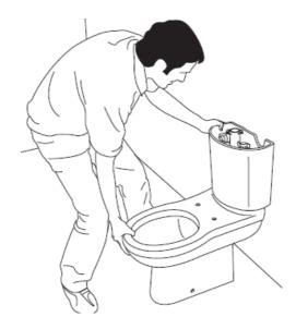
Position the assembled close coupled WC in the desired position, align with the preexisting water and waste provision and level accordingly.
