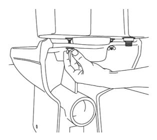
Locate the wing nuts and washers, and screw these onto the threaded bar until they are finger tight. This will secure the cistern to the pan.
