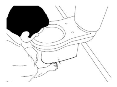
Carefully mark around the base of the pan, also mark a parallel line to show the position of the side fixing holes.
