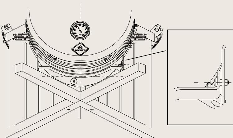
Throughout following Step 11 and Step 12, please centralize front band ⑧ and adjust it to fit the Kamado body as much as possible from time to time.
