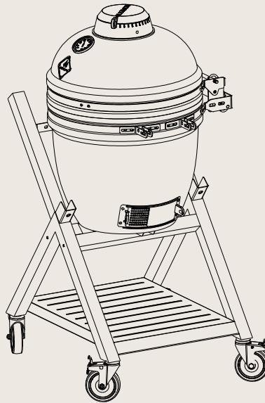
Place Kamado body onto the trolley supporting beams (2) centrally, with inlet air vent towards the right direction. Due to the weight of this grill, we highly recommend two people to perform this task!
