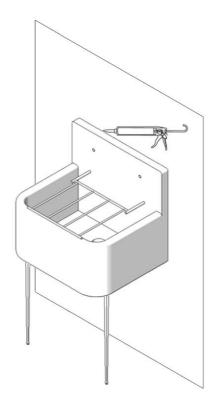
Run a bead of silicon around the outer perimeter of the cleaners sink.
