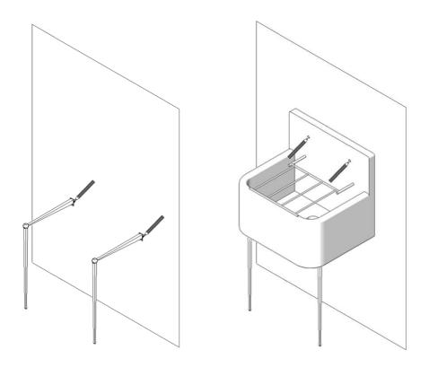
Using the measurements place the legs in position, mark, drill, plug and secure with suitable fixings, then place the cleaners sink ontop of the legs, mark through the screw holes and again drill plug and secure with suitable fixings.
