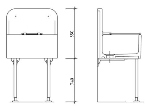
Take the measurements of the cleaners sink and leg-set and allow for provisions for a waste under the sink and water supply for pillar taps or similar above the sink.
