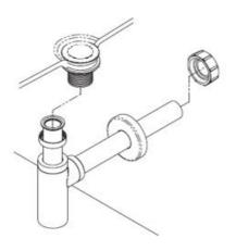
Install the trap and connect the waste pipe to the outlet in the wall
