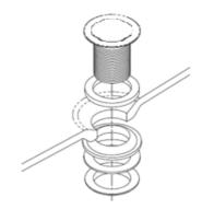
Install the waste into the cleaners sink and tighten.
